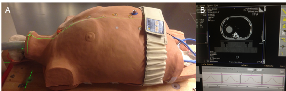
Fig. 10: Phantom set-up for 4D CT and phase assignment: (A): phantom placed on a treatment table, left: tube connected to the ventilation system, right: belt with load cell for respiration measurement, (B): display for phase assignment, lower part shows the breathing cycle and the grey squares represent the same phase.
